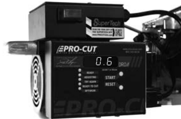
| This display of final compensation equals .0006"
