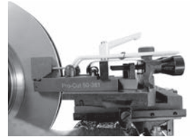
The chip deflector reduces vibration and must be used on EVERY cut.
