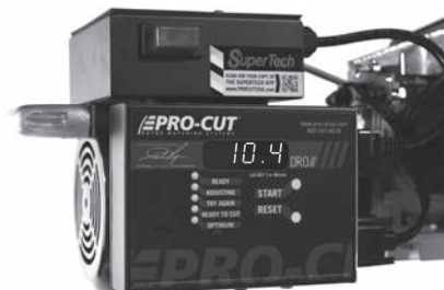
| This value represents hours and tenths of an hour that the motor has run.
