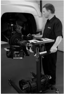
STEP 4. Technician sets cut depth.
